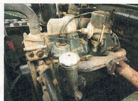
Military spec 2.5-litre turbodiesel powered the 40th (left), while the 80in ambled along with 1.6 petrol
