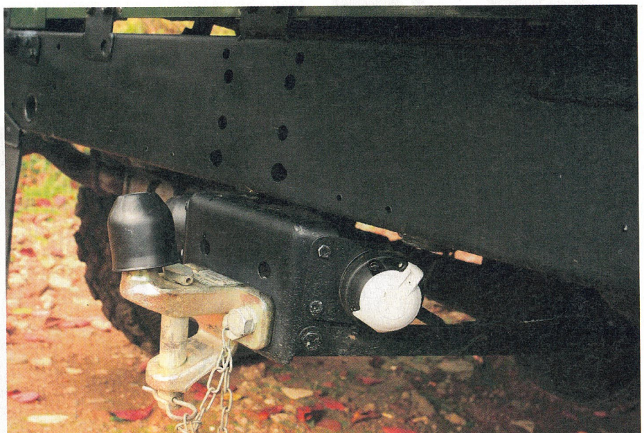
Series 1 agricultural hitch with PTO outlet (above); 40 years on, PTO still exists but original hitch has gone
