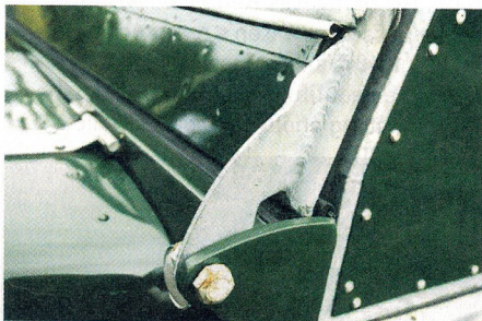
Left: The hinges on the 40th Ninety's windscreen (below) allowed it to fall down flat as featured on the Series 1 80in (left)
