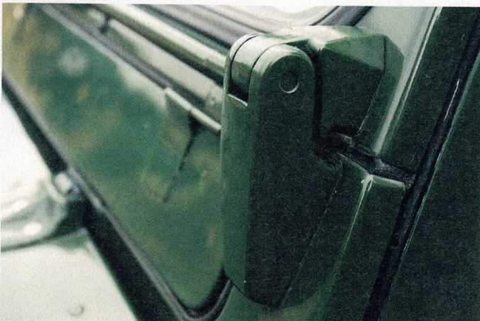
Left: The hinges on the 40th Ninety's windscreen (below) allowed it to fall down flat as featured on the Series 1 80in (left)
