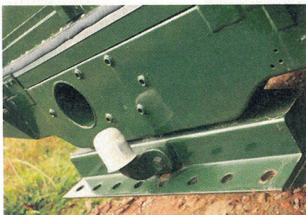
Series 1 agricultural hitch with PTO outlet (above); 40 years on, PTO still exists but original hitch has gone
